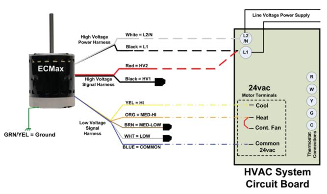
**Rotation** is determined automatically the first time the motor is operated. It is important to operate the motor for the first time in the HVAC system. Do not bench test the motor. The first time the motor is operated the following sequence should be recognized:
